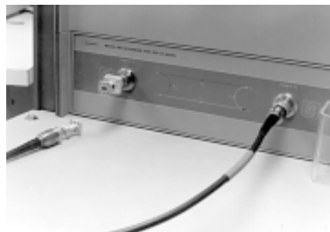
U233E and 8009B Test Port Adapters on an Anritsu 3611 Reversing Test Set
